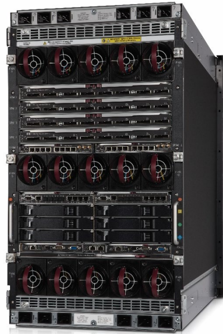
HPE Superdome 2 enclosure back
