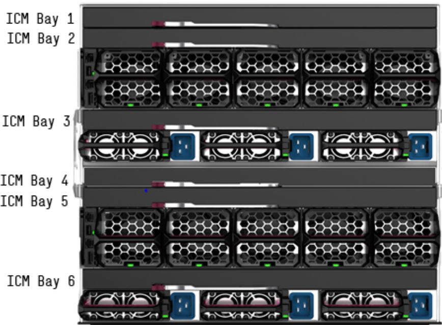
HPE Synergy 12000 Frame - Rear View
